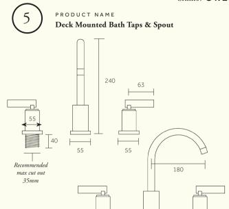
Dimensions in mm (300mm connector hoses supplied)
