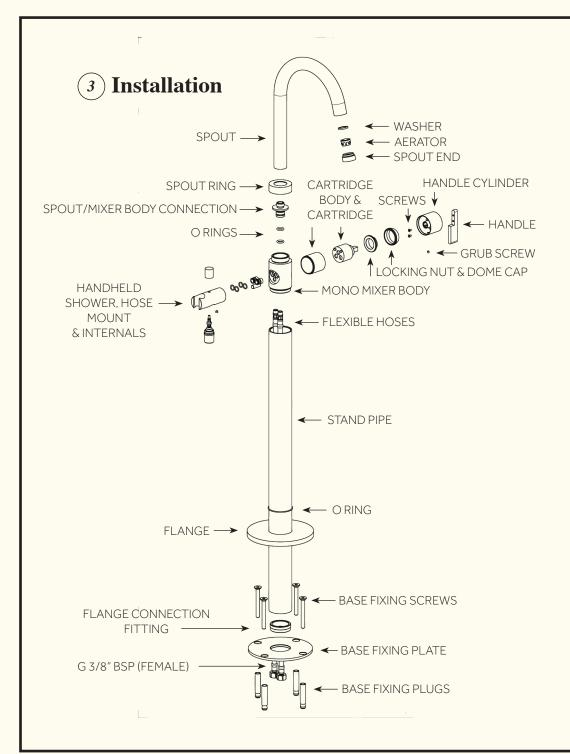
First shut off your water heating system, then with your mains stop cock closed, open the lowest Cold and Hot taps in the house and allow to run until the cold storage tank and pipes are empty (the hot storage cylinder always remains full). Fitting isolating valves to inlet feeds to recommend for ease of maintenance.
