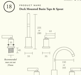
Dimensions in mm (300mm connector hoses supplied)
