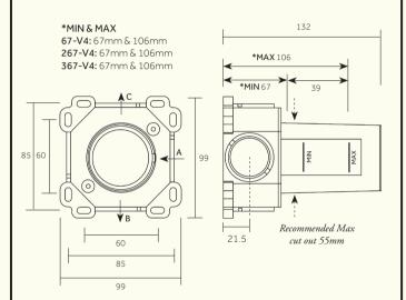
A: G 3/4" WATER INLET B: G 3/4" WATER OUTLET C: G 3/4" WATER OUTLET
