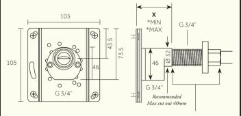
IMPORTANT NOTE: The Thread of the Shower Arms which are pairing with this Internal Part should be cut at the opposite end to where the Olive is installed. Max cut out 40 mm.
