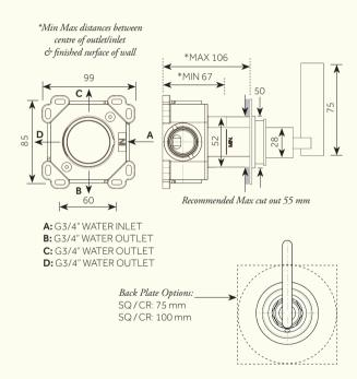
For min/max operating pressures, flow rates (Litres/min) and connection specifications, please see reverse for details.
