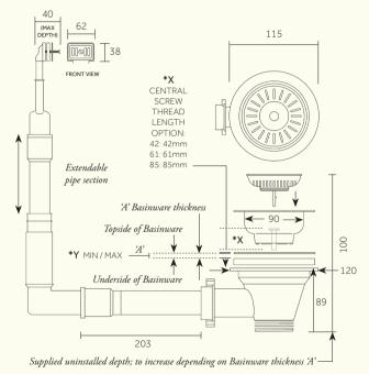
\*Y MIN & MAX VARY DEPENDING ON CENTRAL SCREW INSTALLED:
