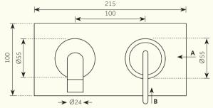
A: 3/4" Cold Water Inlet B: 3/4" Hot Water Inlet
