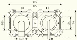
A: 3/4" Cold Water Inlet B: 3/4" Hot Water Inlet
