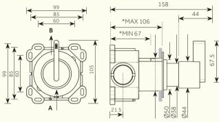
A: G3/4" WATER INLET B: G3/4" WATER OUTLET Recommended Max
