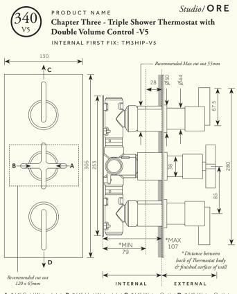
A: 3/4" Cold Water Inlet B: 3/4" Hot Water Inlet C: 3/4" Water Outlet D: 3/4" Water Outlet
