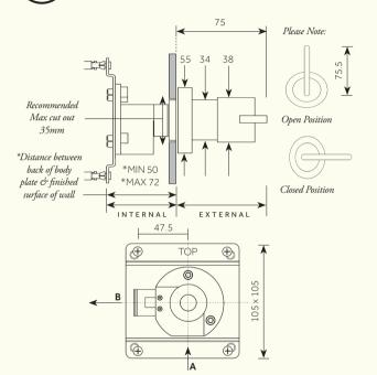
A: G1/2" or 1/2" NPT Water Inlet B: G1/2" or 1/2" NPT Water Outlet
