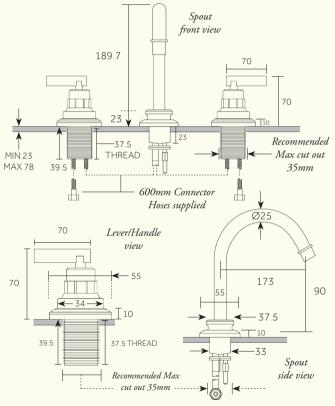
Dimensions in mm. See reverse for Flow Rate & Connection Specifications.
