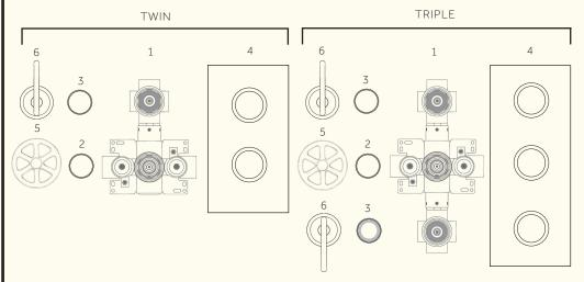
1 Main Thermostatic Shower Valve Body with Diverter Valve (and a CD Valve for the Triple Body). 2 Brass Temperature Body Sleeve. 3 Brass Control Sleeve. 4 Brass Concealing Plate. 5 Brass Thermostatic Control Handle. 6 Brass Flow Control Handle.
