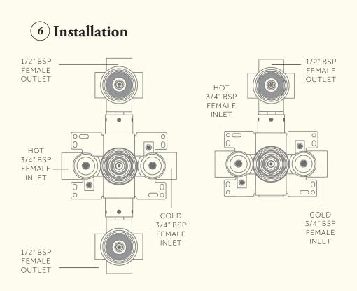
*Twin Valve:* The hot inlet of the valve must be connected to the hot pipe work. The hot inlet of the valve will be marked. When installed correctly the outlet will be facing up.
