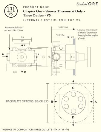
A 3/4" Cold Water Inlet B 3/4" Hot Water Inlet C 3/4" Mixed Water Outlet D 3/4" Mixed Water Outlet
